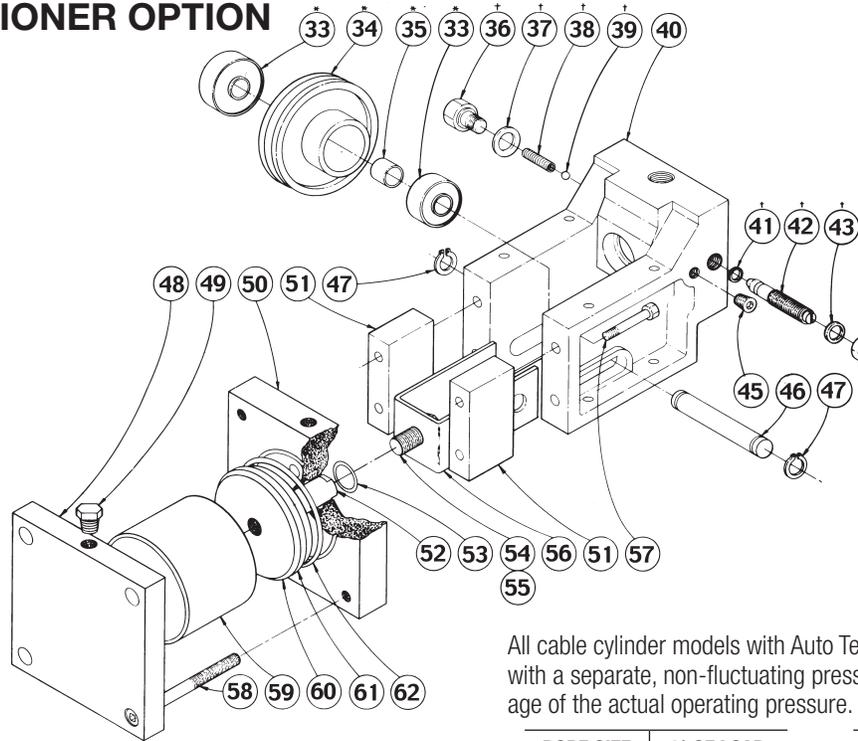
All cable cylinder models with Auto Tensioner units should be plumbed with a separate, non-fluctuating pressure source which is a set percent-age of the actual operating pressure.
