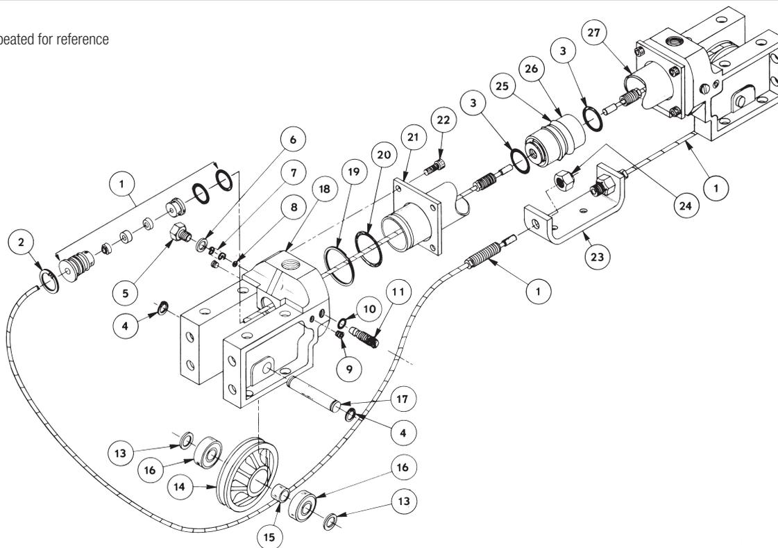
5. Disconnect Cable Assembly (1) from Piston (26) and pull back through the Head assemblies (18) with their gland seals to remove them.
